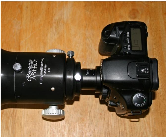
If the observer intends to connect the camera to a telescope, then a T-Mount and an adapter sleeve are essential as can be seen in Fig 4.
